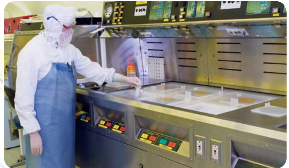
The DDL provides access to a toolset that can produce innovative detectors or bulk micro-machined MEMS devices. Shown here is the wet sector bench for solvents and corrosives.
