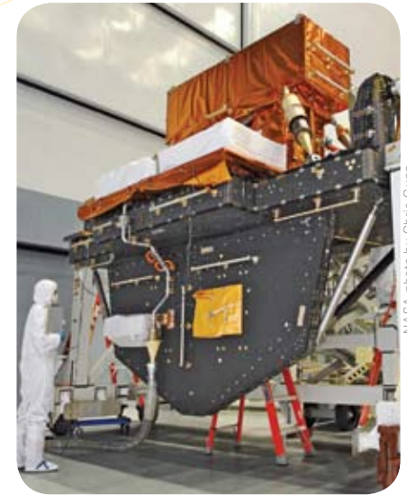
The shuttle's new lightweight carrier, composed in part with TMC, transported the new instruments for SM4.
