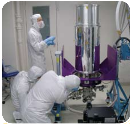
The DCL consists of several laboratories, including class 100 and 10,000 clean rooms for testing contamination-sensitive detectors and subsystems. It is used to perform complete optical and electrical characterizations of large-format detector arrays operating in the ultraviolet, visible, and infrared spectrums.
