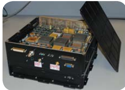
The Navigator GPS technology, part of the RNS system, flew for the first time on SM4.
