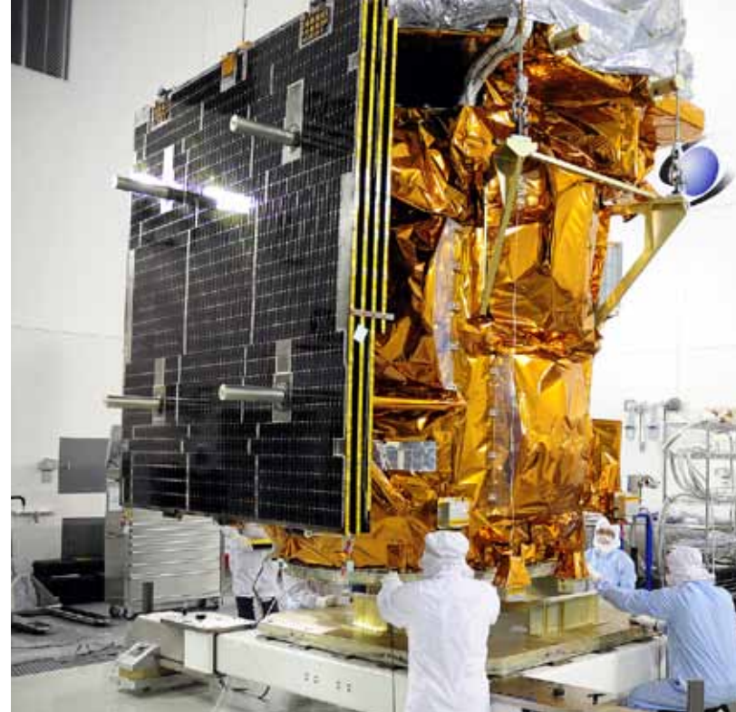
The Operational Land Imager (covered with white Tedlar insulation) and the Thermal Infrared Sensor (covered in gold foil) mounted on LDCM.
