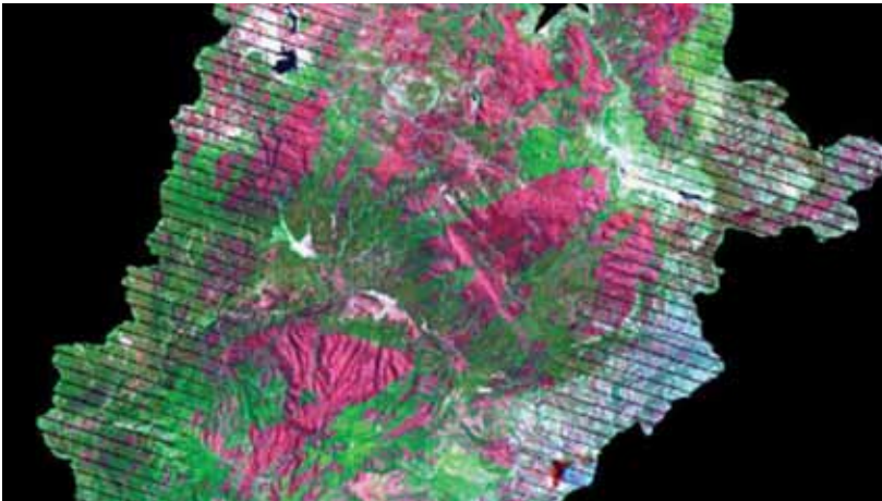
Landsat 7 image of a forest fire in Arizona. Purple represents heavily burned areas. —PHOTO BY NASA
